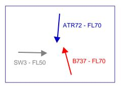
Because the controller is occupied with the resolution of another conflict, the B737 is instructed, late, to descend to FL60 when the aircraft are slightly less than 5 NM head on.
