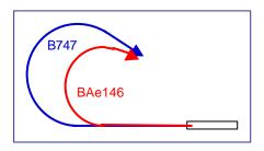
The controller detects the conflict and provides the B747 with traffic information about the BAe146. The pilot replies "we are passing 6000 feet". Then, the controller instructs the BAe146 to "stop climb flight level 60", advising the pilot that a B747 is "1000 ft above climbing". However, two elements have not been taken into account:
