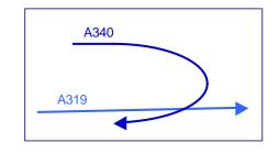
When passing through FL100, the A340 is turned to the right by the departure controller. At the same time, the A319 is cleared by mistake by the en-route controller to climb to FL210, which induces a conflict with the A340. The en-route controller detects the conflict and instructs the A319 to stop climb at FL100. The A319 pilot replies that he has already passed FL100 and that he is descending back to FL100.
