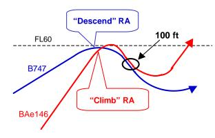
Because the BAe146 pilot did not follow his "Climb" RA, the B747 deviated by 1200 ft. However, despite this large vertical deviation, the B747 pilot reported that the two aircraft passed "very, very, very close" (i.e. 100 ft and 0.5 NM).
