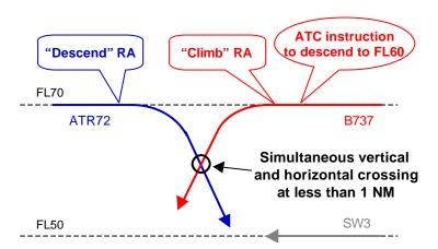
The ATR72 pilot immediately informs the controller that he has a "Descend" RA using the standard phraseology. However just after, the controller repeats to the B737 the instruction to descend to FL60 for avoiding action.
