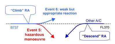
received a coordinated "Descend" RA, which was correctly followed by the pilot. The vertical separation achieved was the vertical deviation of the descending aircraft ft **PLUS** the 100 achieved by the B737.
