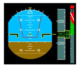
However, an RA display on both the EADI and the vertical speed tape could improve the interpretation by flight crews of "Adjust Vertical Speed" RAs. and other types of RA. This figure shows a possible combined RA display on both the EADI and the vertical speed tape.
