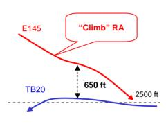
In this event, the high risk of collision resulting from an undetected altimeter setting error was resolved by TCAS, even though the pilot of the E145 did not achieve the vertical speed required by the RA.
