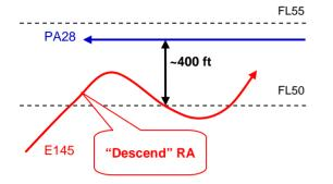
As a result of following the "Descend" RA, the E145 passed about 400 ft below the PA28. Simulations indicate that without TCAS the separation between the aircraft would have only been about 100 ft and 0.04 NM.
