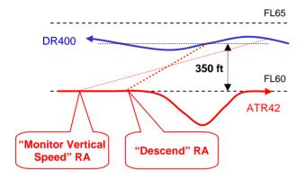
Subsequently, the RA is strengthened into a "**Descend**" **RA** when the vertical separation between the aircraft becomes less than 350 ft. The pilot follows the RA and descends to FL57 before climbing back to FL60.
