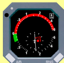
5 seconds after the "Adjust Vertical Speed" RA
