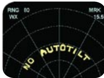
TYPICAL AUTOMATIC TILT FAULT INDICATION
