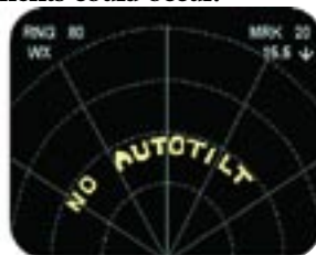
TYPICAL AUTOMATIC TILT FAULT INDICATION
